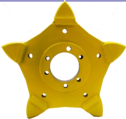
LOG SPROCKET 5-TOOTH Made From 1" Plate Hardened Steel Wider Chain Rests Welded in Hub CNC Machined Heat Treated Bushing Required
