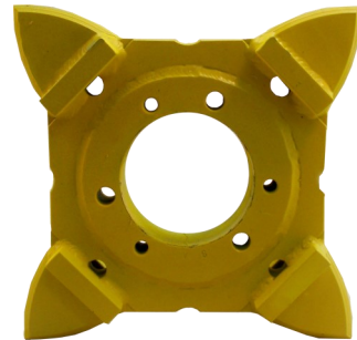
LOG SPROCKET 4-TOOTH Made From 1" Plate Hardened Steel Wider Chain Rests Welded in Hub CNC Machined Heat Treated Bushing Required
